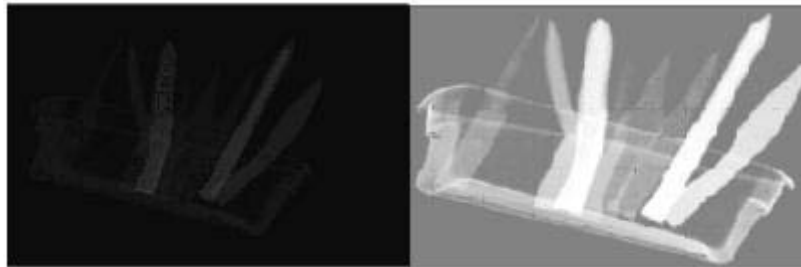
Fig. 8. Original image ( left ) and the image after histogram equalization ( right ). Tomado de [7].
